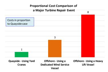
reconnected to the mooring lines. Repair operations quayside are significantly less costly and less risky than undertaking repairs at site with a floating crane, or even in sheltered coastal water with a floating repair vessel. Major repair costs near shore or offshore are between 3 to 8 times more costly than completing repairs quayside (including towing of the platform from site to quayside to reinstalling at site).
